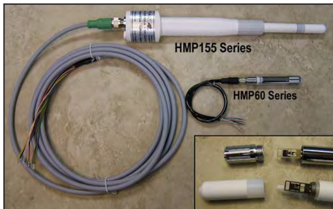
225-HMP155A & 225-HMP60A Relative Humidity & Temperature Sensors
