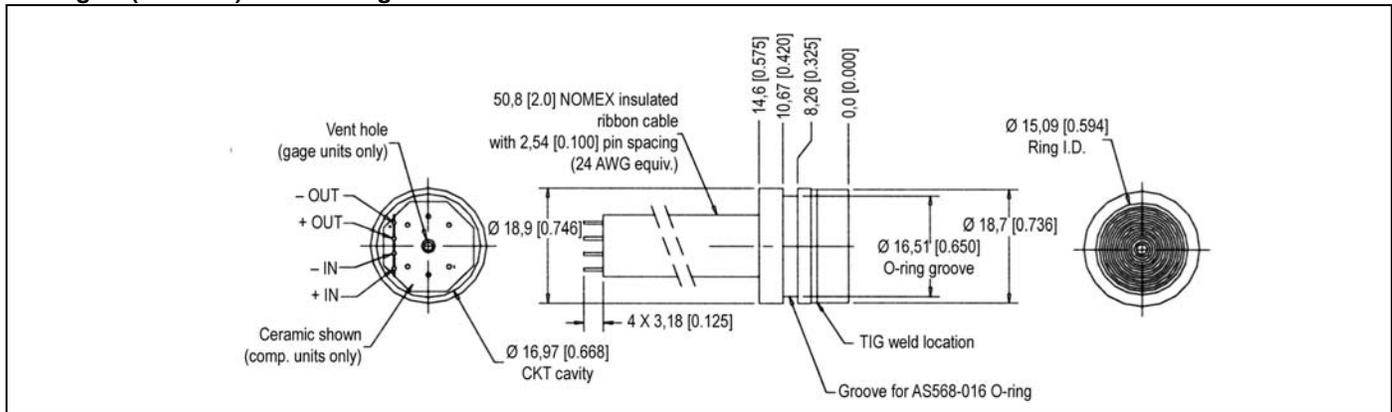
**Note:** Non-concentricity effects at the diaphragm weld area may cause runout of up to  $\pm 0.006$  in between the upper and lower portions of the sensor body. (It is recommended to use a counter bore to mate with this device to allow for this non-concentricity).
